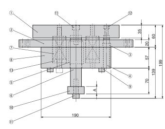
\*1 To lock out in closed position, put a 5mm-spacer between Lifter Plate (①) and Base Plate (②) and fasten by a bolt. The spacer and the bolt are not included.
