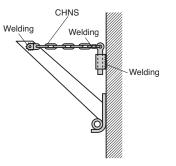
The chain-set described as CHNS is to be fixed onto the lower die and the scrap chute.
