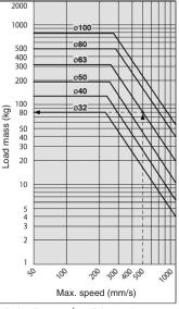
Cylinder diameter  $\phi$ 63, if the maximum speed of 500 mm/s, load mass is 80 kg.
