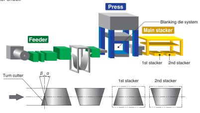
One unit of the turn blanking die can produce trapezoid blank sheets. One press stroke can produce one blank sheet.
