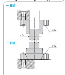
Tapped hole for lifting bolt is drilled on the guide bushing.
