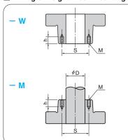
Tapped hole for height block mounting is drilled on the guide bushing.
