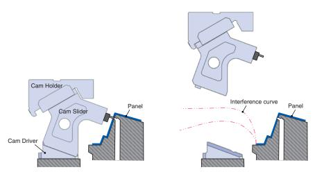
Cam position during panel processing.
